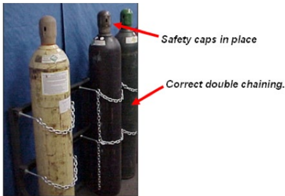
Figure 9.1—Gas Cylinders Stored Correctly
