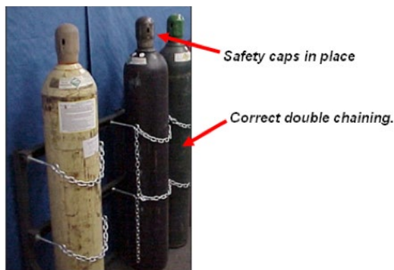
Figure 9.1—Gas Cylinders Stored Correctly
