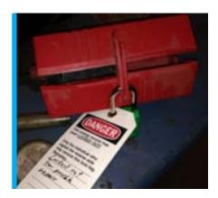
Lockout/tagout/blockout (LOTO) is a method of preventing equipment from being set in motion and endangering workers. Failure to properly isolate and de-energize energy sources can be fatal. Compliance with the University's LOTO policy is mandatory for your protection and the protection of others.
