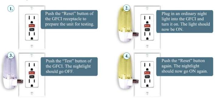
The nightlight should go out when the "Test" button is pushed. If the light does not go out, then the GFCI may have been improperly wired or damaged and does not offer shock protection. In this case, contact a licensed electrician to check the GFCI and correct the problem.
