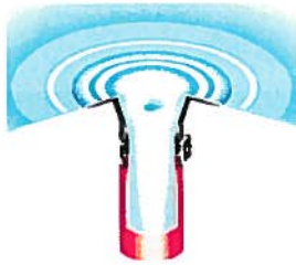
Air and water enter a gravity outlet
