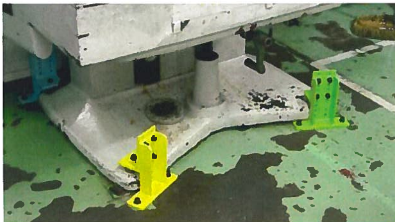
Production equipment anchored to the floor
