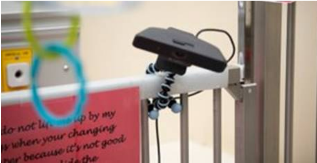
Figure 3. Flexible tripod and webcam mounted to crib
