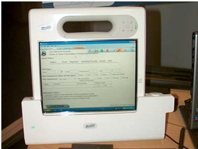
A tablet for doctors and nurses: the Motion Computing C5 Mobile Clinical Assistant. Clad in a durable white casing with a built-in handle and a splash-proof seal around the LCD screen, the C5 has an Ingress Protection (IP) rating of 54, which means that it can withstand a light liquid spray and wipe clean — ideal for a device that will require regular disinfection. <sup>iii</sup>
