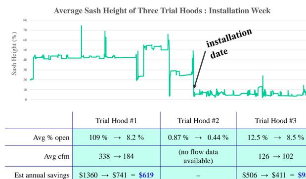
**Figure 3:** (top) timeplot of sash heights averaged across all three trial labs, (bottom) tabulated estimated savings per year
