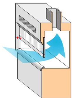
**Figure 1:** Diagram showing basic fume hood flow. Front sash height dictates amount of air sucked from room.
