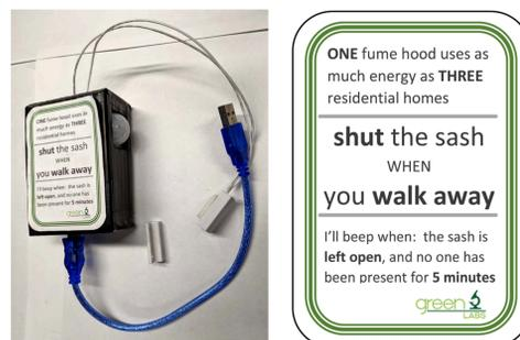
**Figure 2:** (left) constructed MASH device per MIT Green Labs instructions<sup>2</sup> and (right) UCSD info label.
