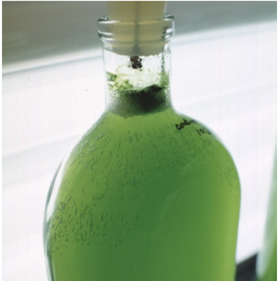
Hydrogen bubbles forming inside a flask of sulfur- and oxygen-deprived green algae.
