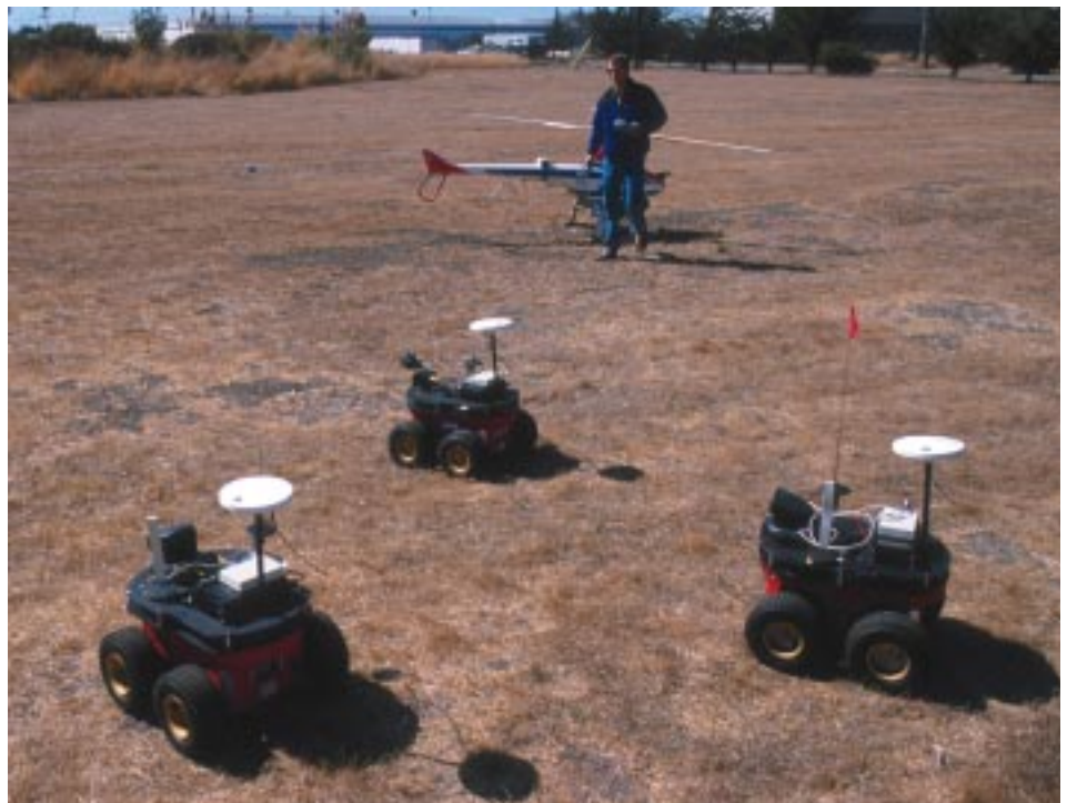
Three ground robots wait in front of the robot helicopter. The white platters are GPS antenna. The vehicles are also equipped with optical cameras or laser rangefinders. Each vehicle functions autonomously and as part of a wireless network that connects all the vehicles together.
