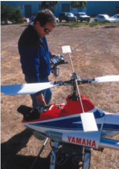
Senior development engineer Ron Tal adjusts a robotic helicopter. Based on a remote-controlled agricultural helicopter, this robot has been designed to land autonomously on a pitching platform that models the deck of a ship in a severe storm.
