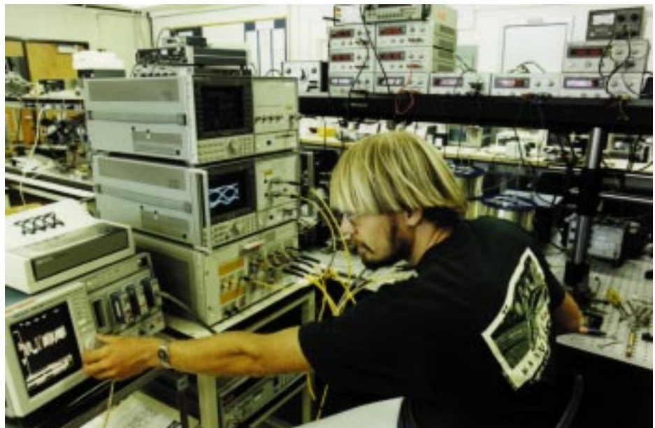
The communication system being tested here can transmit at the 30 gigabit level—30 billion bits per second.
